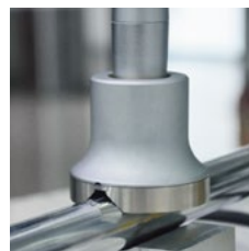
Measuring hardness of nut with Standard Probe Protector
